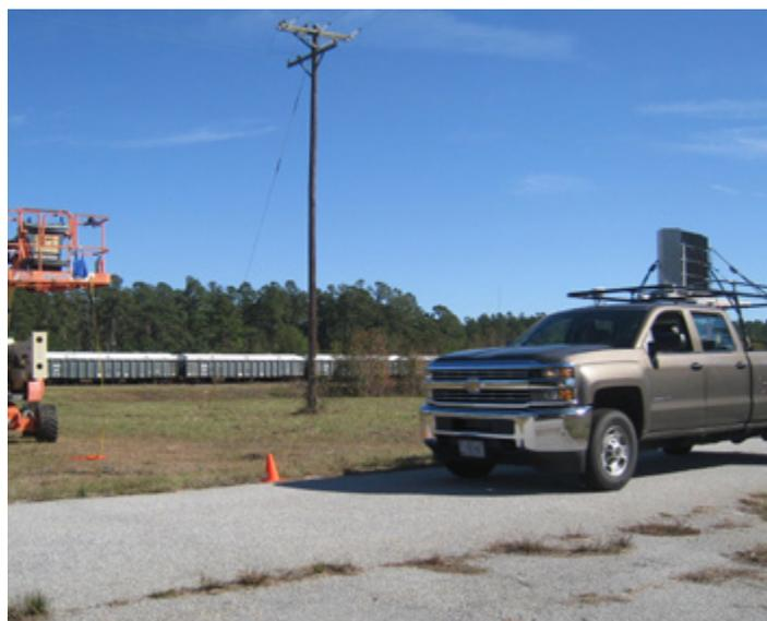
*Detection testing commences at the SRS railyard. Vehicle-mounted radiological monitoring equipment attempts to detect and identify radioactive sources in a variety of freight transport scenarios.*
