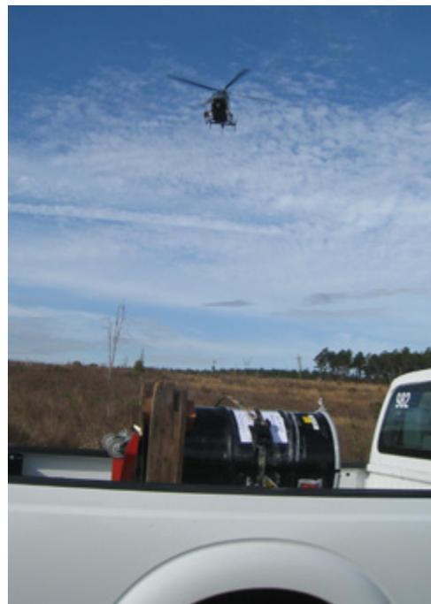
*A helicopter equipped with radiological detection equipment evaluates a test container from several hundred feet away.*
