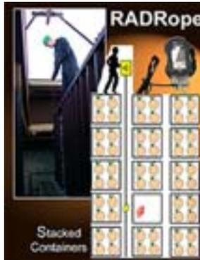
The RadRope™ system can be used in a straight line, a curved line, or an angled line. For example, the system can be mounted on a frame through which items of interest can be passed. The length of the RadRope™ system can be easily customized for different uses.
