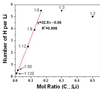
Plot of Number of hydrogen atoms per lithium atom vs The mol ratio of  $C_{60}:Li$ . An ratio of 1:6 ( $C_{60}:Li$ ) achieved the highest  $H_2$  capacity (5.0%).
