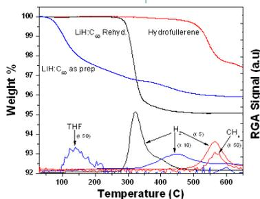
TGA-RGA comparison of the 3<sup>rd</sup> desorption Of the  $LiH:C_{60}$  (6:1) composite (as prepared-blue and Rehydrated-black) and hydrofullerene (red). The materials were hydrogenated at 350°C under 105 bar  $H_2$ .
