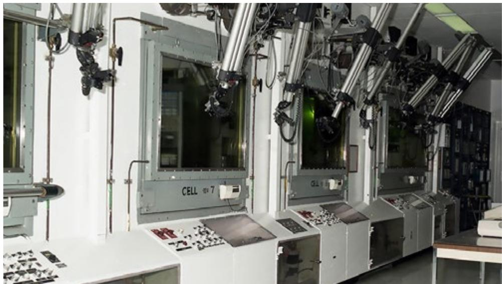
*The Shift Operating Base inside the PuFF Facility was a clean area that allowed operators to use remote manipulators to work with material inside the cells.*
