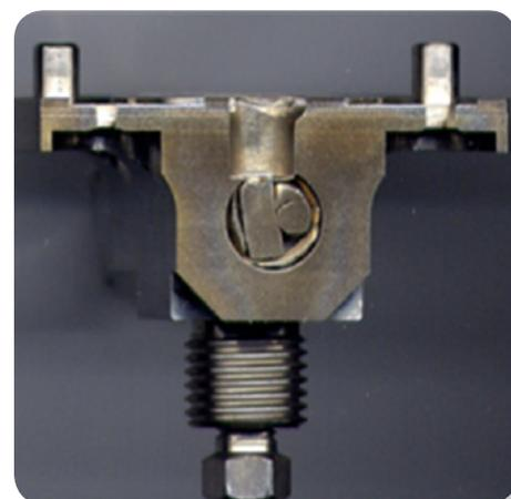
*Debris trap showing pinch weld sheared by piston*
