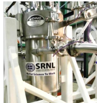
Centrifugal contactor that mixes the waste stream with the solvent
